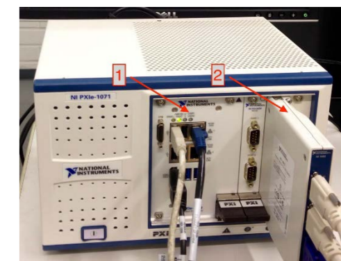
PXI System (1. RT-Controller, 2. Camera Link module connected to FPGA module).
