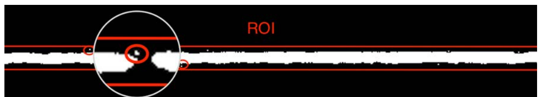
Threshold image with unwanted particles
