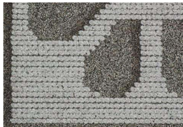
Fig. 1. Digital camera (left) and optical microscope (right) images of Ekspla logo marked on silicon wafer. The marking resolution was 50 μm in both transverse x and y directions.
